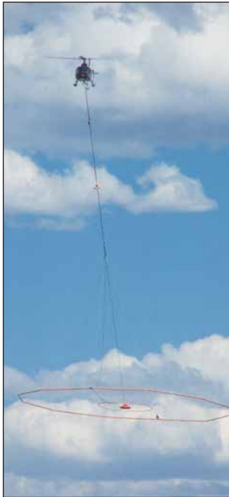
Canadian company Geotech makes passes over the SPNRD with its 'spider web' array. The system might give scientists a look at geology as far as 600 feet below the earth's surface.
